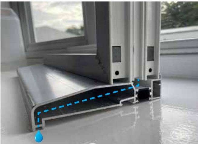
On some door configurations, the drainage will be 'face drained' through the bottom of the frame. On most configurations, drainage will go through the sill as illustrated. Hence the importance of not drilling through this chamber as water would not be drained accurately and could enter the property.
