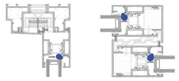
After installation of the glass and correct packing you can now fit the glass perimeter foam (grey foam tubing supplied in the box). This is simply a push in foam that helps to increase the weather protection of the doors. Cut to the length required (glass size + 100mm) and push into the gap between the glass and the sash as illustrated in the pictures. It is normal to start at the top corner and work your way around.
