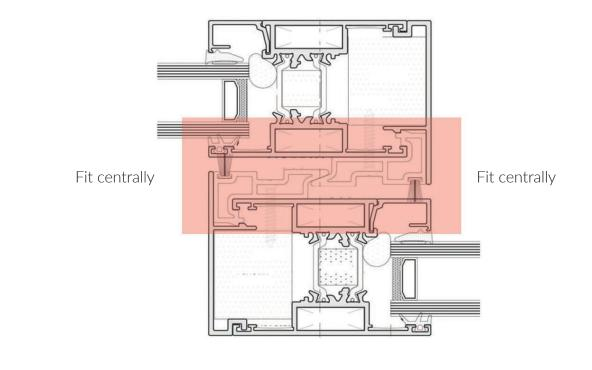
Apply silicone in centre hole after installation
