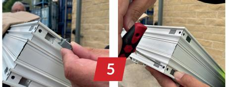
Once this is done, insert the cleat blocks as illustrated. Following this, fix the cleat blocks with a 3mm allen key (not supplied).
