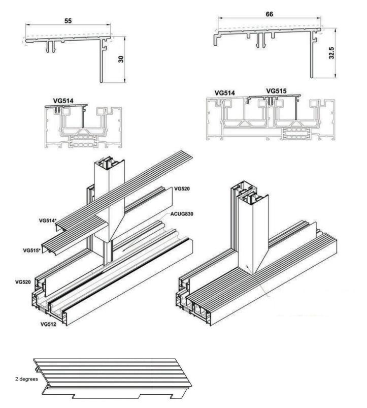
Supplied cut to a 2 degree angle. The bottom tread will have notches for the drainage. The notches fit around the frame closers (see FRAME CLOSERS page).
