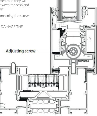
Please note that if you need to adjust the wheel for height then it is easier to do before fitting the anti-lift / covers as they must be removed to gain access to the adjuster screw.
