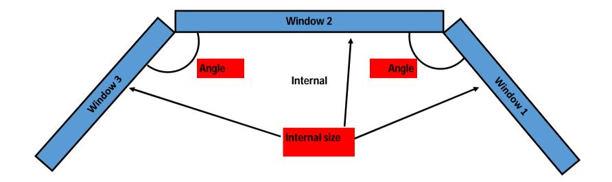
Internal sizes and angles required Quickslide will make the deductions for the bay poles Welded sill available on request
