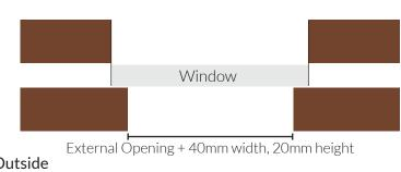
Important - Check that the internal width and height are larger than external.
