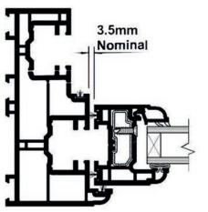
Check gap between both sashes and outer frame.
